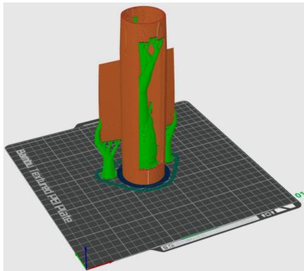
We used Bambu Studio in combination with the Bambu A1 3D printer to fine-tune our prints by adjusting key settings such as wall loops, rectilinear infill, outer wall speed, and tree supports.
