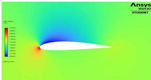
The NACA 2412 provide the best lift to drag ratio and pressure difference when compared with other airfoils.
