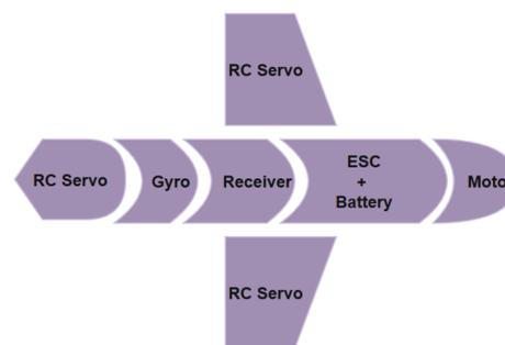
Each location for the electrical components were housed taking the center of gravity into account.
